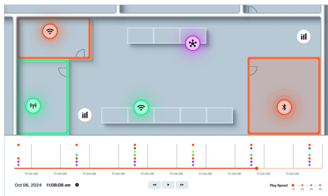
Figure 4: Bastille UI screenshot showing accurate real time location on a floor plan of cellular, Wi-Fi and Bluetooth devices
